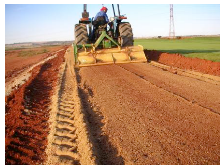
Rotovator used for mixing & tilling
